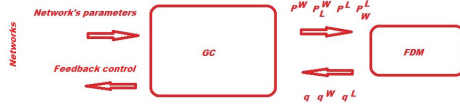
Fig. 1. Coordination between GC and FDM involves passing parameters and solutions to the optimization
