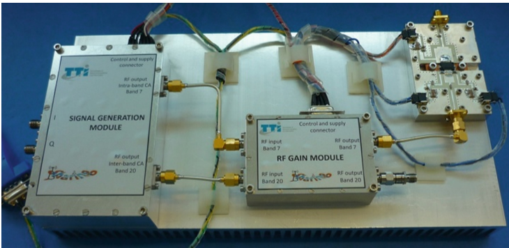
Fig. 8. Picture of the reconfigurable RF front-end prototype.
