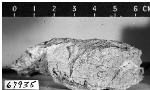
Sample 67935, a 0.23-kg chip from a shatter cone on the House Rock at Station 11.
