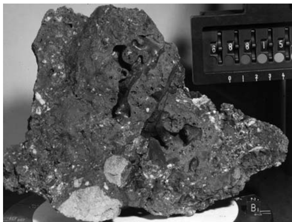
Sample 68815, a 1.83-kg dark-matrix breccia chipped from the vesicular boulder at Station 8.
