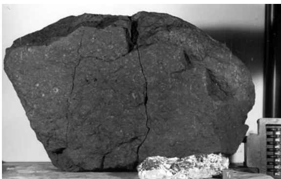
Sample 70215, an 8.11-kg very finely grained gabbro that Jack Schmitt collected near Challenger for the reason that it was typical of the valley floor unit.
