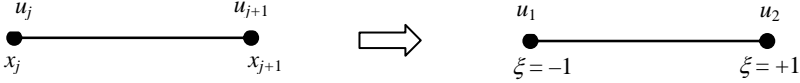
Figure 3.2. Mapping of an element, defined on x \in [x_j, x_{j+1}] , to a canonical element defined on \xi \in [-1, +1] . The known functions u_j and u_{j+1} are mapped as u_1 and u_2 in the \xi coordinate system
