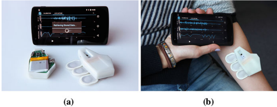
Fig. 6.17 (a) Wearable muscle fatigue tracking system, showing the Android application and the wearable device, (b) Complete muscle fatigue tracking system, showing the Android application and the wearable device attached on a user
