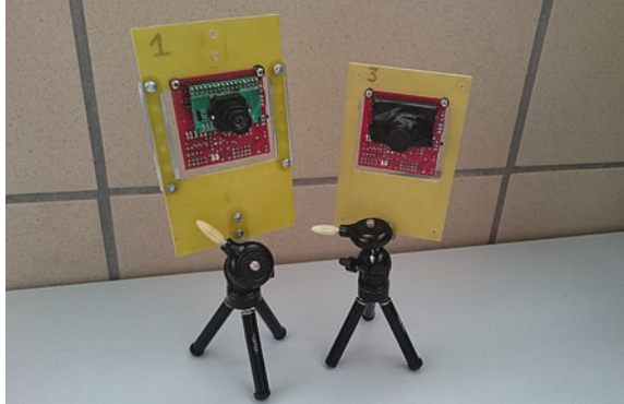
Fig. 2.3 Nodes of the WCN: each node is composed of a CMUcam3 module and a WSN node
