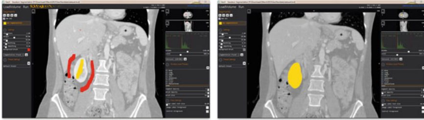
Fig. 4.1 Segmentation method: with only a foreground stroke for the kidney ( yellow ) and two background strokes for the surrounding organs ( red, left image ), an initial segmentation of the kidney is obtained ( right image ). This segmentation can be further refined with more strokes
