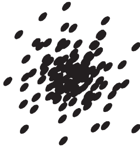
Figure 2.6.2. Schematic image of a just-resolved double source obtained with a very short exposure time.
