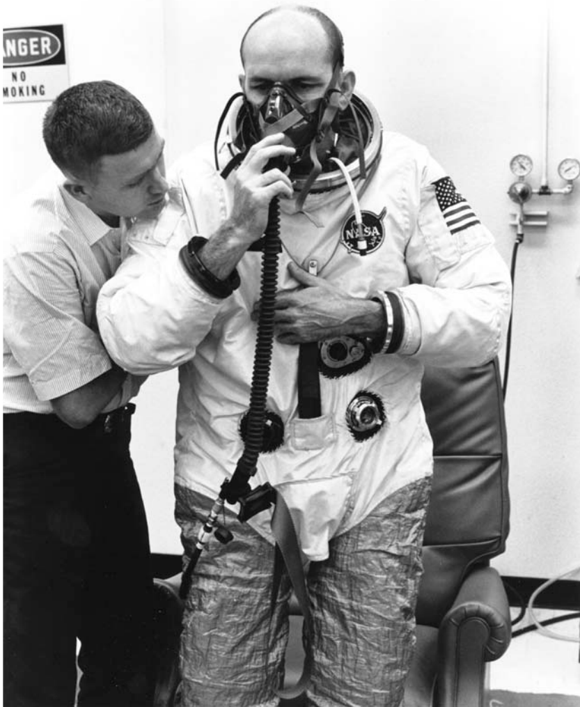
33. Wearing a Gemini EVA space suit fitted with thermal protection material on the legs, Ed Givens prepares to undertake an altitude chamber test. This heavily insulated suit was designed specifically for use with the Astronaut Maneuvering Unit. (NASA)
