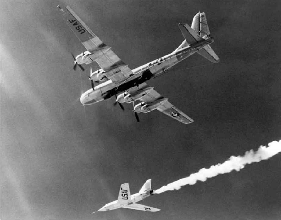
13. The Bell Aircraft X-2 drops away from its Boeing B-50 mother ship in this 1955 photo. Lt. Col. Frank "Pete" Everest piloted the X-2 on its first unpowered flight on August 5, 1954. Everest made the first supersonic X-2 flight on April 25, 1956, achieving a speed of Mach 1.40. In July, he reached Mach 2.87, just short of the Mach 3 goal. (NASA photo)
