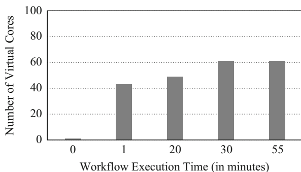
Fig. 2.3 The number of virtual cores in each period of time during the SciPhy workflow execution initiated with a VM [11]
