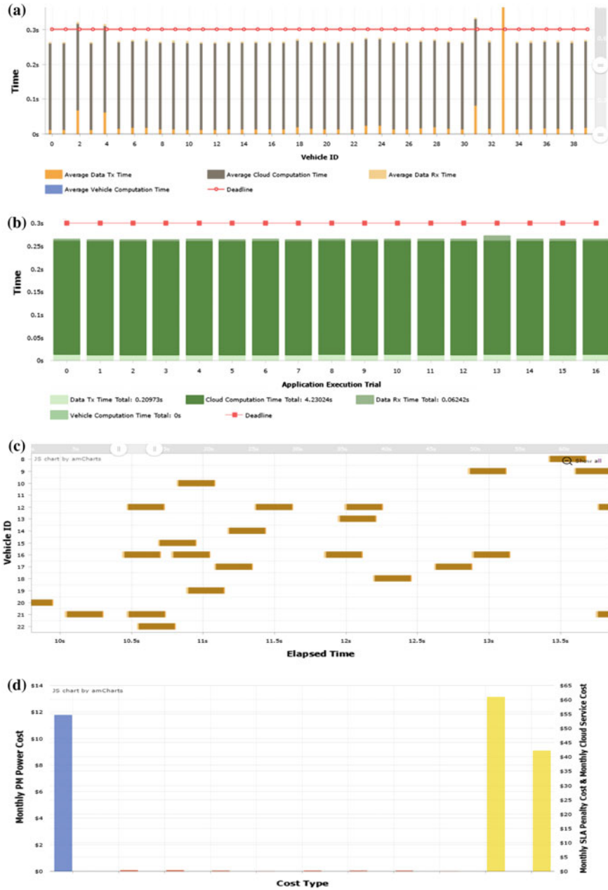
Fig. 4.12 An example of the selected simulation results. a Average service completion time (for all vehicles). b Service completion time (for each vehicle). c Service completion time (Gantt chart). d Monthly profit analysis of the cloud provider. e Handover count. f Average RLC downlink throughput. g Average RLC uplink throughput. h Average downlink SINR. i Average uplink SINR. j PDRC downlink throughput. k PDRC uplink throughput. l Transmitted packet number. m Received packet number. n Transmitted byte size. o received byte size. p Packet loss ratio
