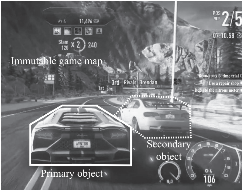
Figure 2.5 Game play showing primary and secondary objects. The game player owns the left car and interacts with the right car. The device closest to the owner of the left car would contain the primary copy of the left car object and a replica of the right car object (courtesy: http://www.metacritic.com ).
