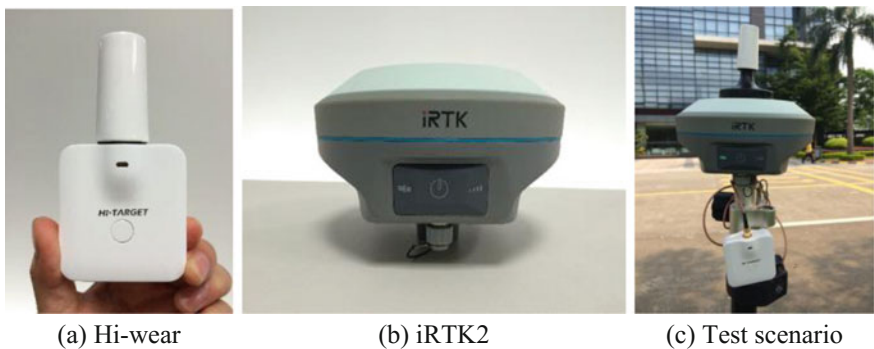
Fig. 6 GNSS devices used in the tests. a Hi-wear b iRTK2 c Test scenario
