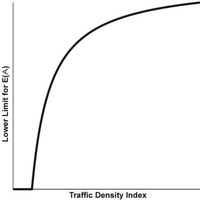
Fig. 3.8 Lower limit of the expectation for the characteristic area of a traffic jam as a function of a traffic density measure. The expected value will be larger than this, and can vary unpredictably, making the estimation of a Macroscopic Fundamental Diagram impossible above the threshold density
