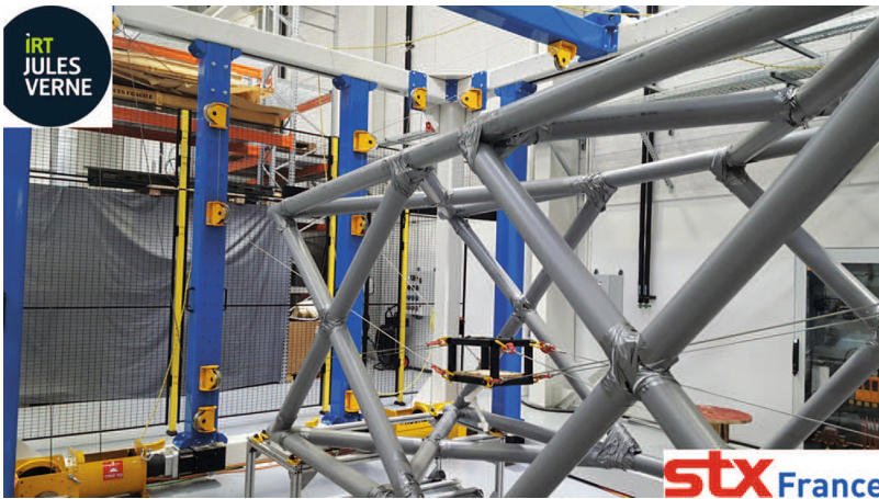
Fig. 1. CAROCA prototype: a reconfigurable cable-driven parallel robot working in a cluttered environment (Courtesy of IRT Jules Verne and STX France)
