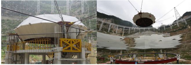
Fig. 5. View of the model cabin (in a left-right order): (1) Model cabin and its harbor; (2) Airborne cabin
