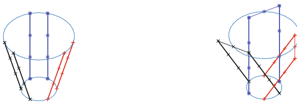
(a) Trivial architecture designed to avoid interference between cables. (b) Architecture inspired by the geometry proposed in [8] for platforms with six actuators and crossing cables.
