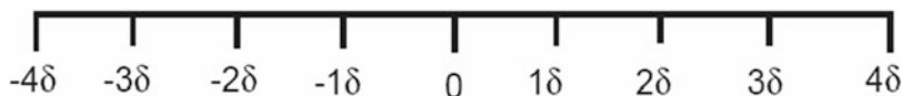
Fig. 2.1 A one-dimensional random walk of particles placed at z = 0 at t = 0 . The particles occupy only the positions 0, \pm\delta, \pm2\delta, \pm3\delta, \pm4\delta
