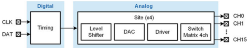
Fig. 4.6 The block diagram of the neural stimulator. The stimulator consists of an analog part and a digital part. The stimulator integrates four independent driving sites, and each site demultiplexes to four channels
