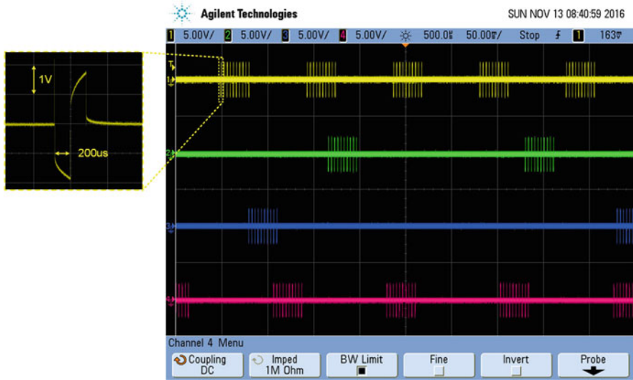
Fig. 4.14 The measured simultaneous stimulation output from four independent channels. The boxed window shows the measurement of a single pulse in high resolution
