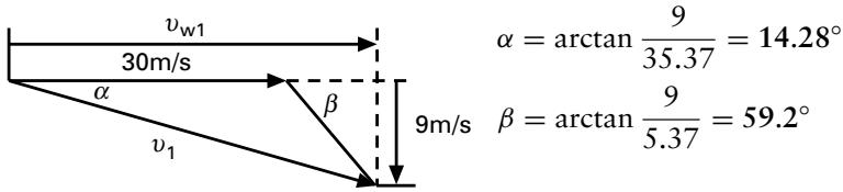
$$\frac{v_1^2}{2g} = \frac{35.37^2 + 9^2}{19.62} \text{ m} = 67.9 \text{ m}$$
