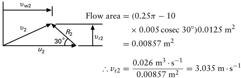
$$v_{w2} = (19.63 - 3.035 \cot 30^\circ) \text{ m} \cdot \text{s}^{-1} = 14.38 \text{ m} \cdot \text{s}^{-1}$$
