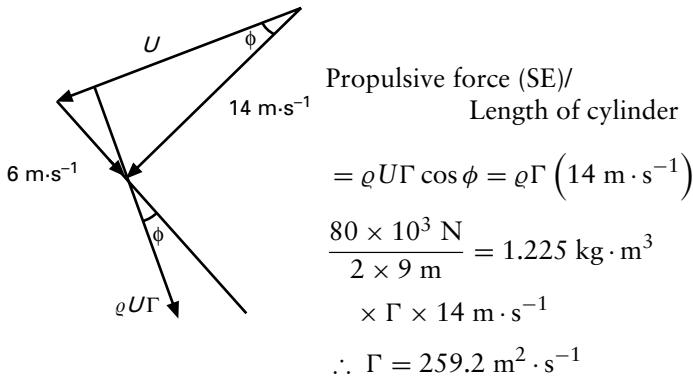
$$\text{But } \Gamma = 0.5 \times 2\pi r \times \omega r = \pi r^2 \omega$$
