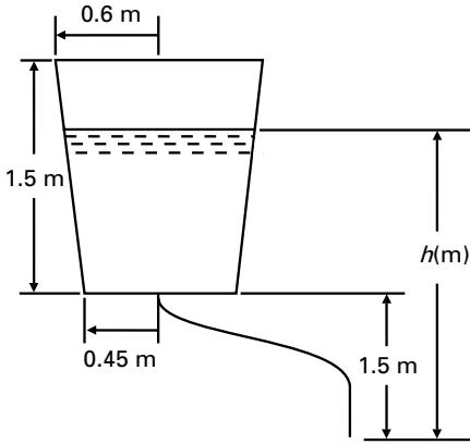
$$\begin{aligned} A &= \pi r^2 \\ &= \pi \{0.45 + (h - 1.5)\}^2 \text{ m}^2 \\ &= \pi (0.3 + 0.1h)^2 \text{ m}^2 \end{aligned}$$
