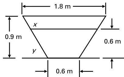
$$\begin{aligned}\frac{x}{0.6 \text{ m}} &= \frac{0.6}{0.9} \\ \therefore x &= 0.4 \text{ m} \\ y &= \sqrt{0.4^2 + 0.6^2} \text{ m} \\ &= \sqrt{0.52} \text{ m}\end{aligned}$$
