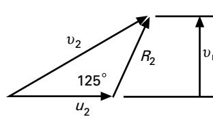
$$\begin{aligned} \tan 55^\circ &= \frac{v_{r2}}{v_{w2} - u_2} \\ &= \frac{0.1508}{D [ (5.15/D) - 83.1D ]} \\ &\quad [\text{metre, second units}] \end{aligned}$$
