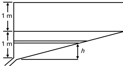
$$\begin{aligned} &\text{For upper, rectangular, portion} - (18 \times 9 \text{ m}^2) db \\ &= 0.9 \frac{\pi}{4} (0.15 \text{ m})^2 \\ &\quad \times 2\sqrt{2gh} dt \end{aligned}$$
