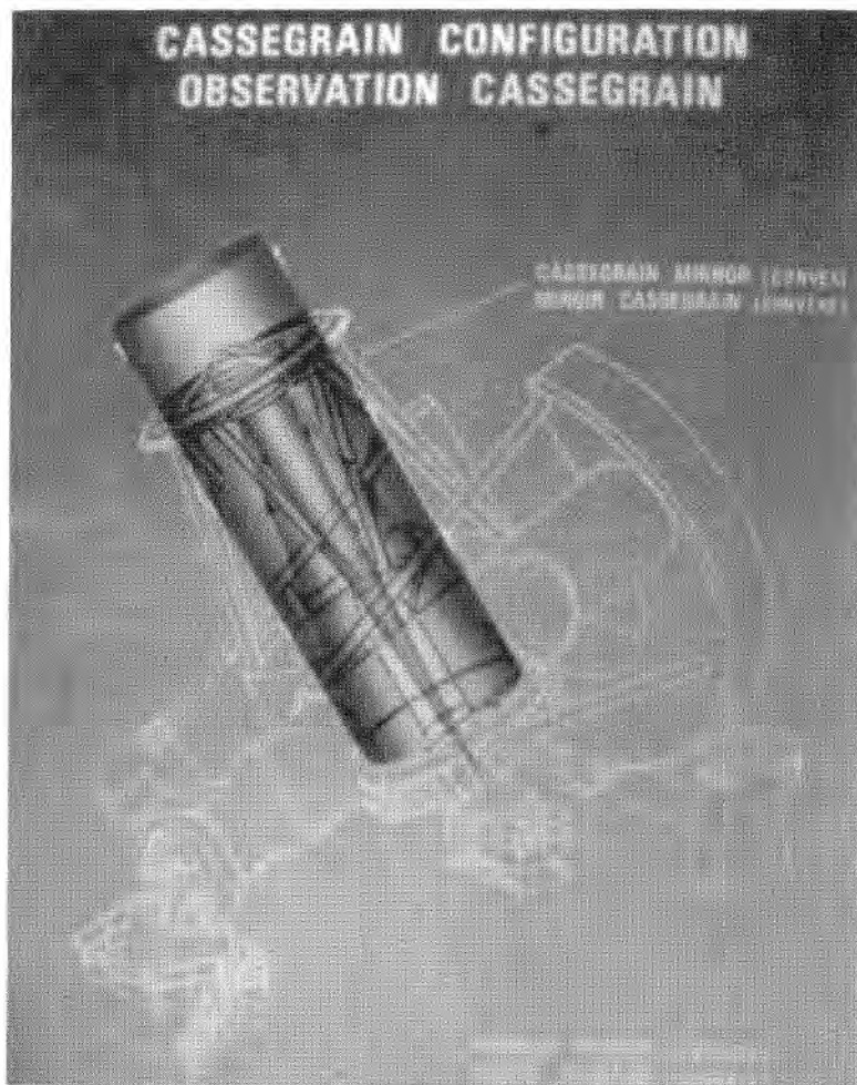
Schematic showing setup for Cassegrain observations. (Courtesy Canada-France-Hawaii Corporation)
