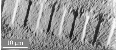
Fig. 2.40. Written longitudinal recording track pattern observed in a magnetic force microscope, displaying the magnetic charges at the transitions. (Courtesy D. Rugar , IBM Research)
