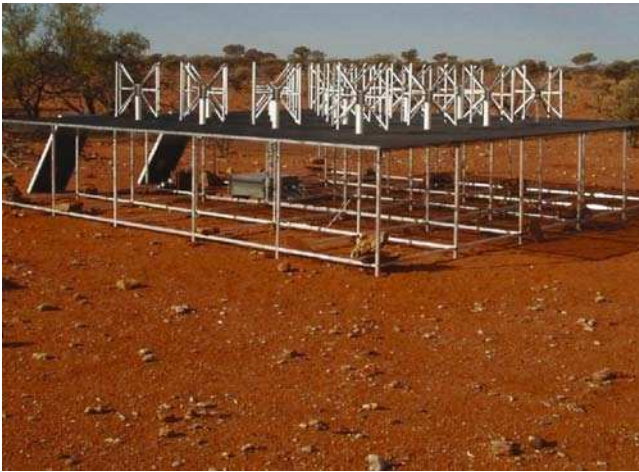
Fig. 55. Prototype of the tile design for the Mileura Wide-Field Array (MWA) in western Australia, aimed at detecting redshifted 21 cm from the epoch of reionization. Each 4\text{ m} \times 4\text{ m} tile contains 16 dipole antennas operating in the frequency range of 80–300 MHz. Altogether the initial phase of MWA (the so-called “Low-Frequency Demonstrator”) will include 500 antenna tiles with a total collecting area of 8000\text{ m}^2 at 150 MHz, scattered across a 1.5 km region and providing an angular resolution of a few arcminutes
