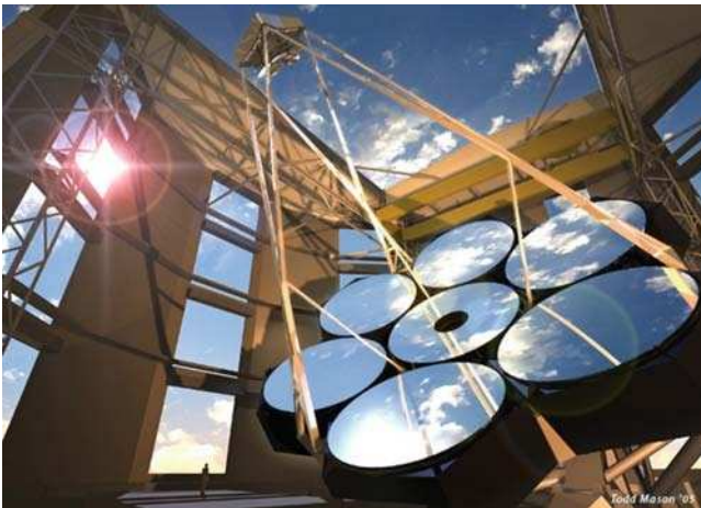
Fig. 5. Artist conception of the design for one of the future giant telescopes that could probe the first generation of galaxies from the ground. The Giant Magellan Telescope (GMT) will contain seven mirrors (each 8.4 m in diameter) and will have the resolving power equivalent to a 24.5 m (80 ft) primary mirror. For more details see http://www.gmto.org/
