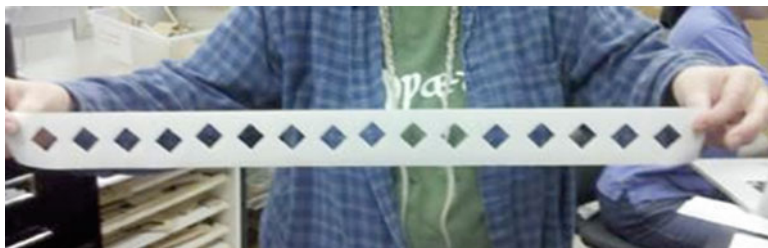
Fig. 18.6 A length of paper tape, spooled by the device in Fig. 18.5, in which a succession of diamond-shaped holes have been cut
