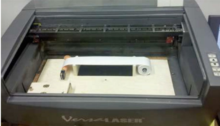
Fig. 18.5 A computer-controlled paper-tape spooler device has been placed on the table of a desktop laser cutter. The basic idea of the device is that it permits users to progressively spool lengths of paper tape that can be cut or engraved by a moving laser. Details of the device’s construction can be found at the Instructables.com website, at: http://www.instructables.com/id/Scrollable-Laser-Cutting-Addition/
