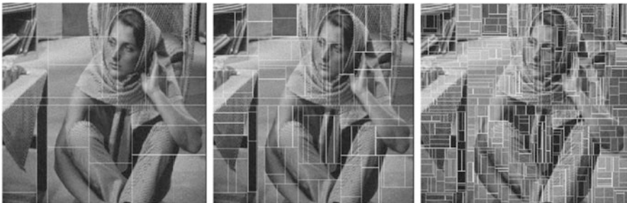
Fig. 17.3 Partition of the image of different size using rpart . The right-hand panel displays the final partition, which is composed of 686 regions
