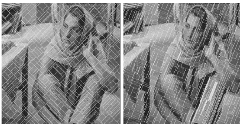
Fig. 17.5 Partition of the image using rotation with angle \alpha = 30 ( left ) and \alpha = -60 ( right )
