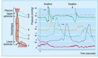
Figure 4.9 Normal recording at oesophageal manometry (horizontal arrows indicate progression of normal oesophageal peristalsis)
