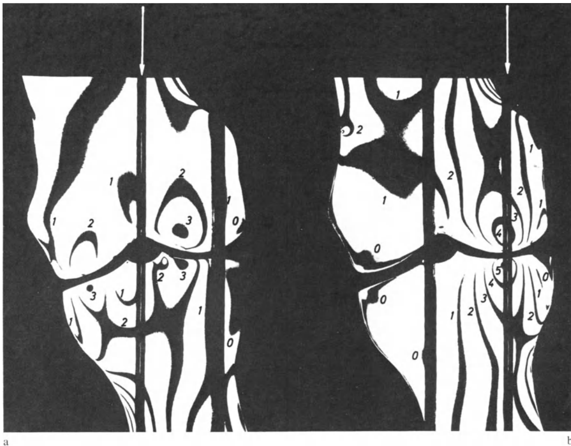
Fig. 129a and b. Isochromatics appearing in a photoelastic model of the femoro-tibial joint supporting a load oblique to the tibial plateaux. (a) Centred load. (b) Eccentric load
