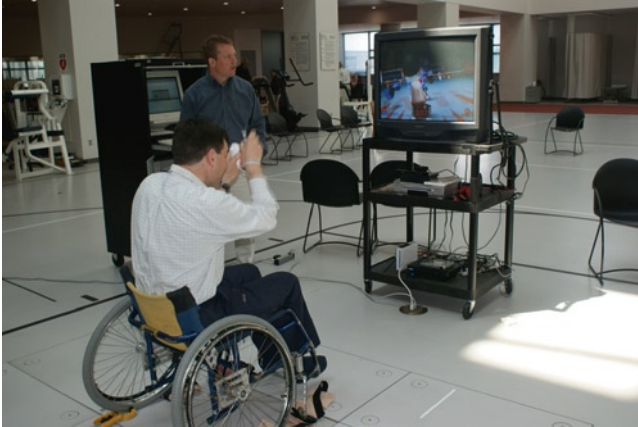
Fig. 7 Wii Boxing in a wheelchair on a force platform
