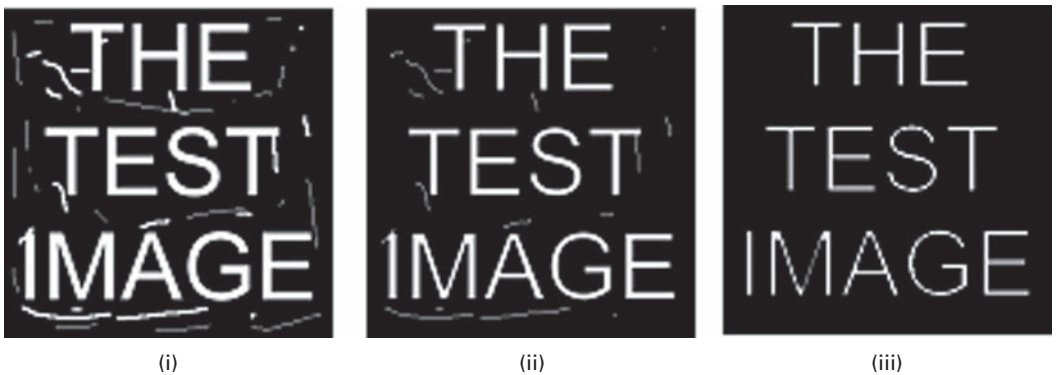
Figure 9.9 (i) Original image; (ii) after a single erosion; (iii) after two erosions.
