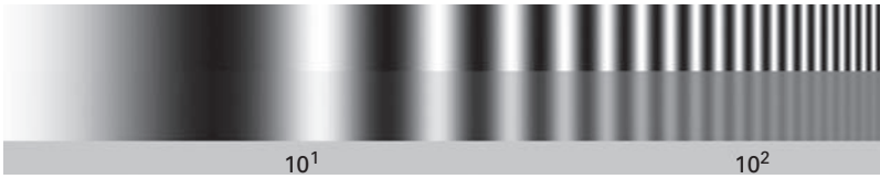
Figure 7.28 (Top) A sinusoidal test pattern of uniform contrast with spatial frequencies from 2 to 200 \text{lp mm}^{-1} and (bottom) the image formed by a certain imaging system. The modulation transfer function of the system drops to 0.5 (50%) at \sim 42 \text{ lp mm}^{-1} and to 0.1 (10%) at \sim 126 \text{ lp mm}^{-1} .
