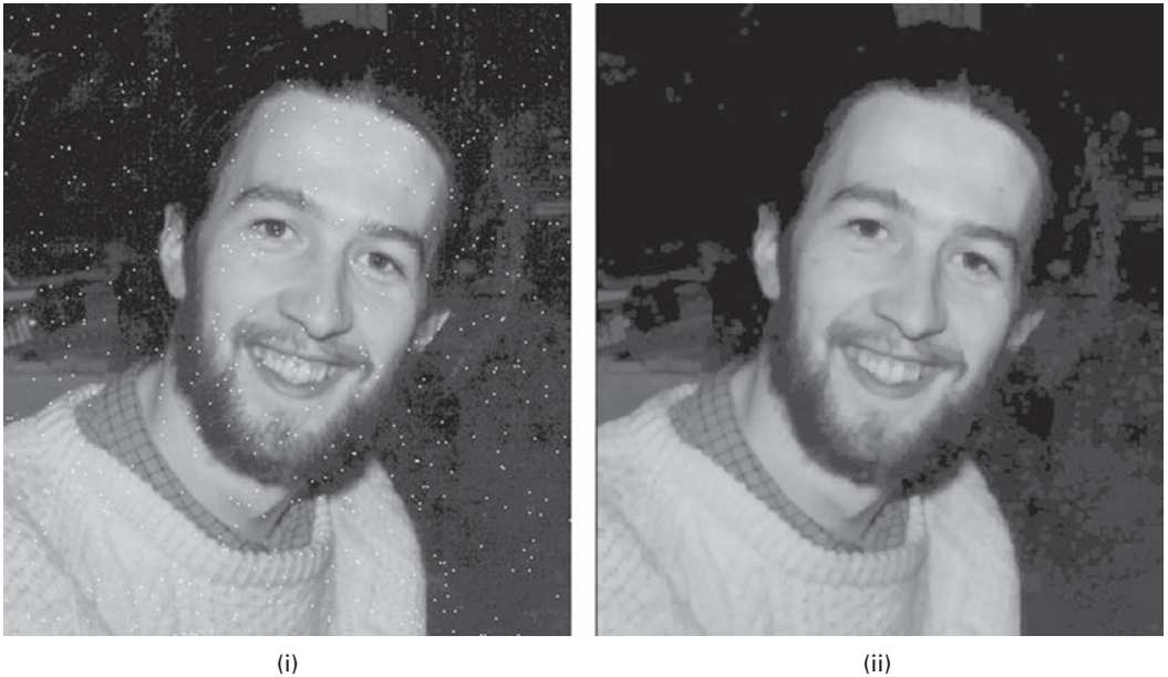
Figure 9.37 (i) Original image with “salt” noise and (ii) after grayscale opening with a flat 3 \times 3 square structuring element.
