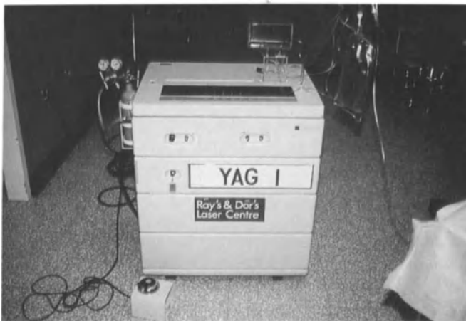
FIGURE 30.7.9. An SLT 100-W Nd-YAG laser.
