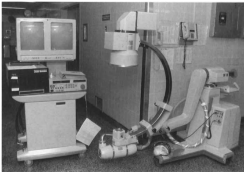
FIGURE 11.3.1. A mobile fluoroscopy unit capable of producing enhanced images and providing hard copies.
