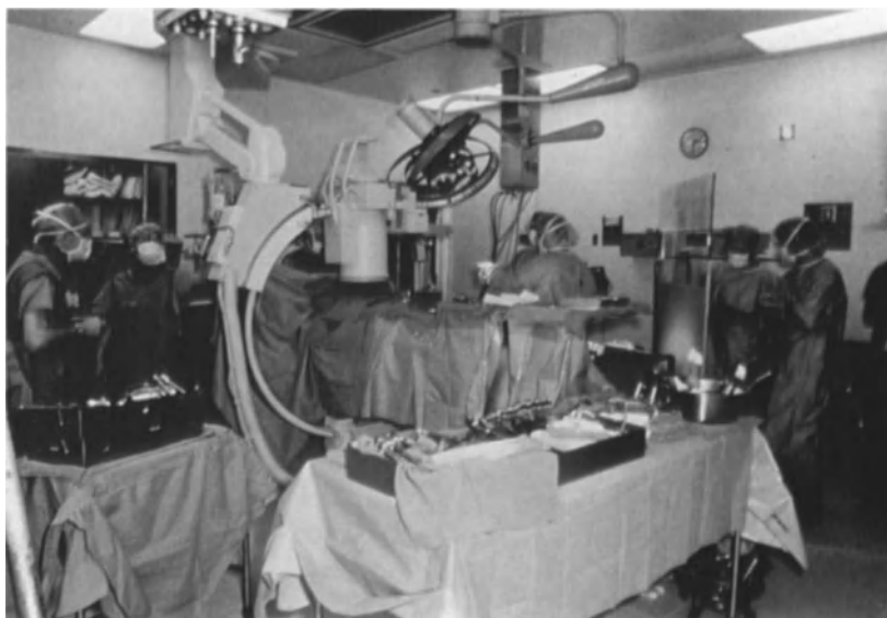
FIGURE 11.3.2. A ceiling-suspended C-arm with coaxial cable audiovisual link to the radiology department provides the surgeon with rapid and efficient cholangiography.
