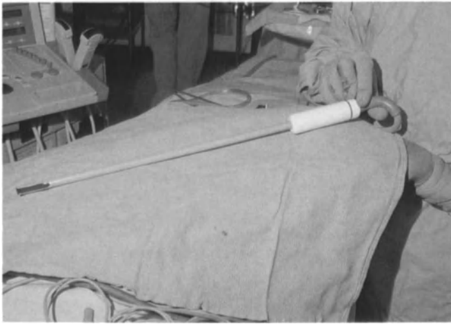
FIGURE 27.1. Prototype Acoustic Imaging laparoscopic ultrasound probe.
