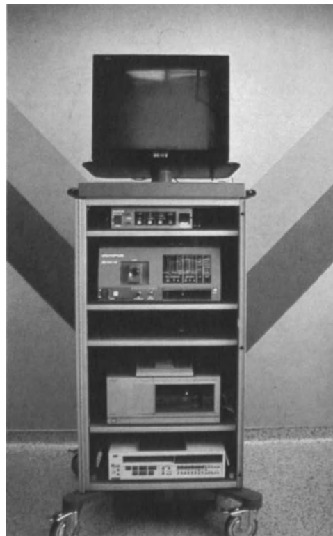
FIGURE 2.1. Typical video set-up, including light source, VCR, and mavigraph.
