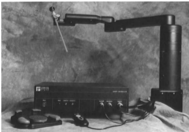
FIGURE 38.6.3. AESOP laparoscopic positioning system. Device accepts real-time input from the surgeon.
