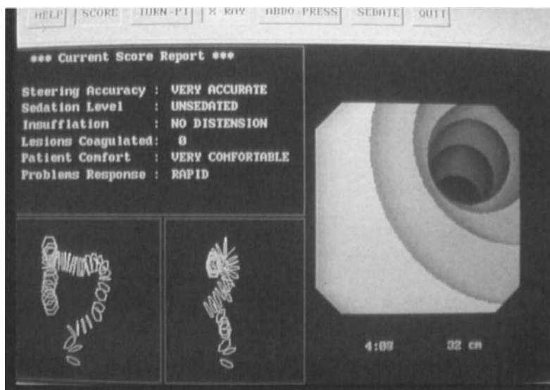
FIGURE 38.4.2. Computer graphic colonoscopy simulation showing Lambertian shading and 3-D modeling of the colon.
