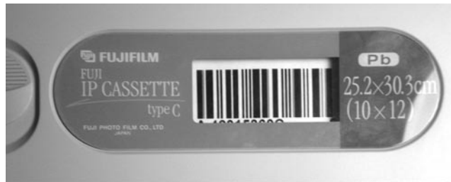
Figure 4-5 Barcode identification labels.
