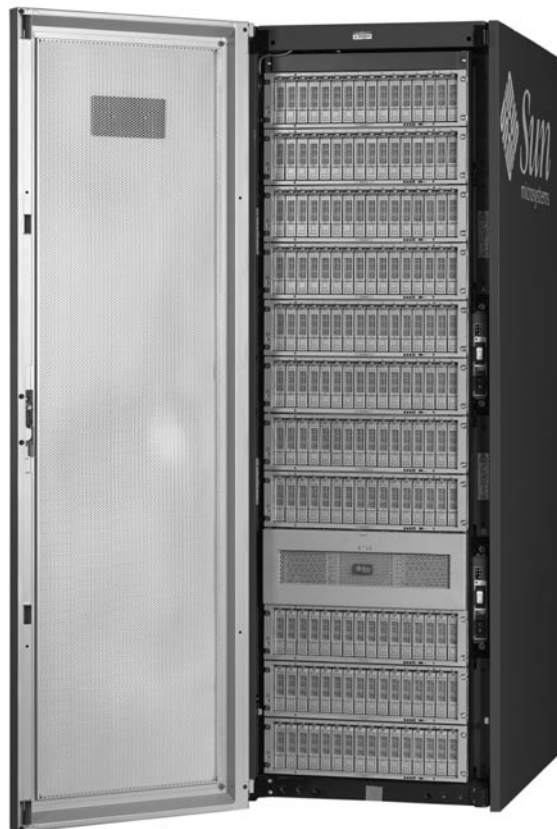
Figure 9-4 A redundant array of independent disks. (Courtesy Sun Microsystems.)
