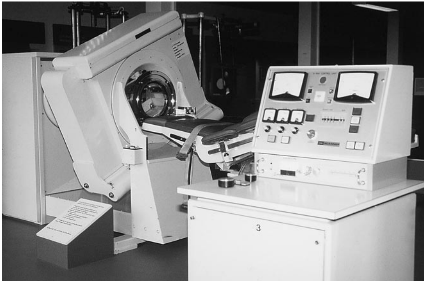
Figure 1-1 First-generation EMI CT unit: dedicated head scanner.
