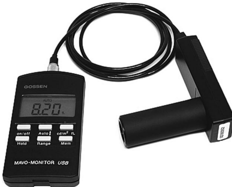
Figure 11-3 A photometer used to measure luminescence.
