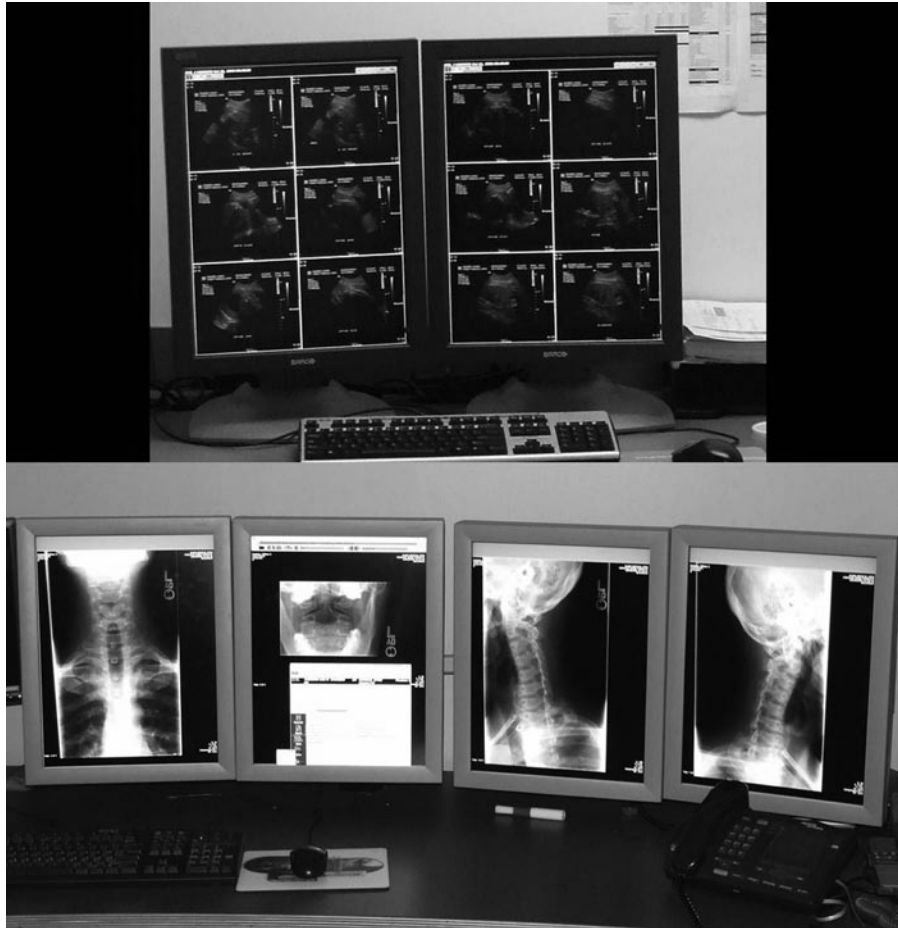
Figure 8-12 A four-bank monitor workstation and a two-bank monitor workstation.
