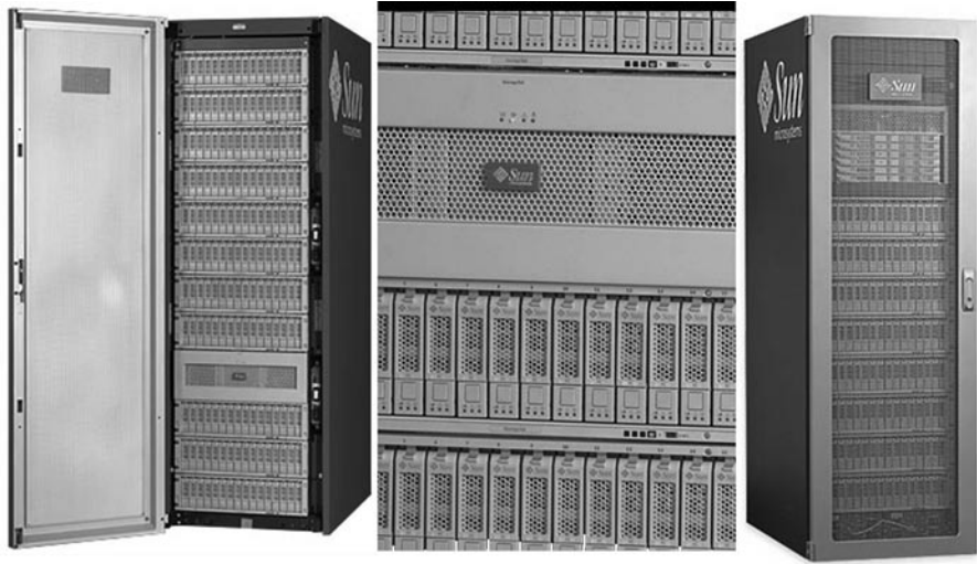
Figure 9-17 Magnetic disk storage used as a long-term archive. (Courtesy Sun Microsystems.)
