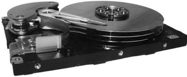
Figure 2-15 Looking inside the hard drive.
