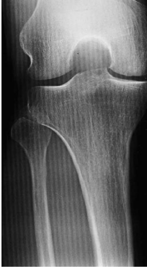
Figure 7-2 Aliasing artifact caused by grid aliasing, also known as the moiré effect. (From Cesar LJ, Schueler BA, Zink FE, et al.: Artefacts found in computed radiography , Br J Radiol 74:195–202, 2001.)
