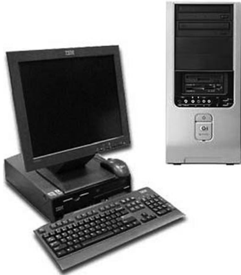
Figure 2-4 The desktop model is pictured on the left, and the tower is pictured on the right.
