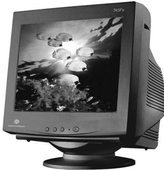
Figure 2-17 Cathode ray tube (CRT) monitor.
