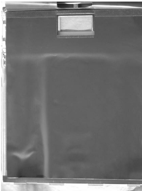
Figure 4-2 Aluminum absorber in cassette.
