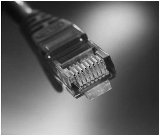
Figure 3-9 RJ-45 jack connected with twisted-pair Ethernet wire.
