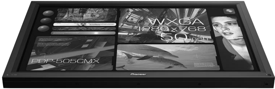
Figure 2-19 Plasma display. (Courtesy Pioneer Inc.)
