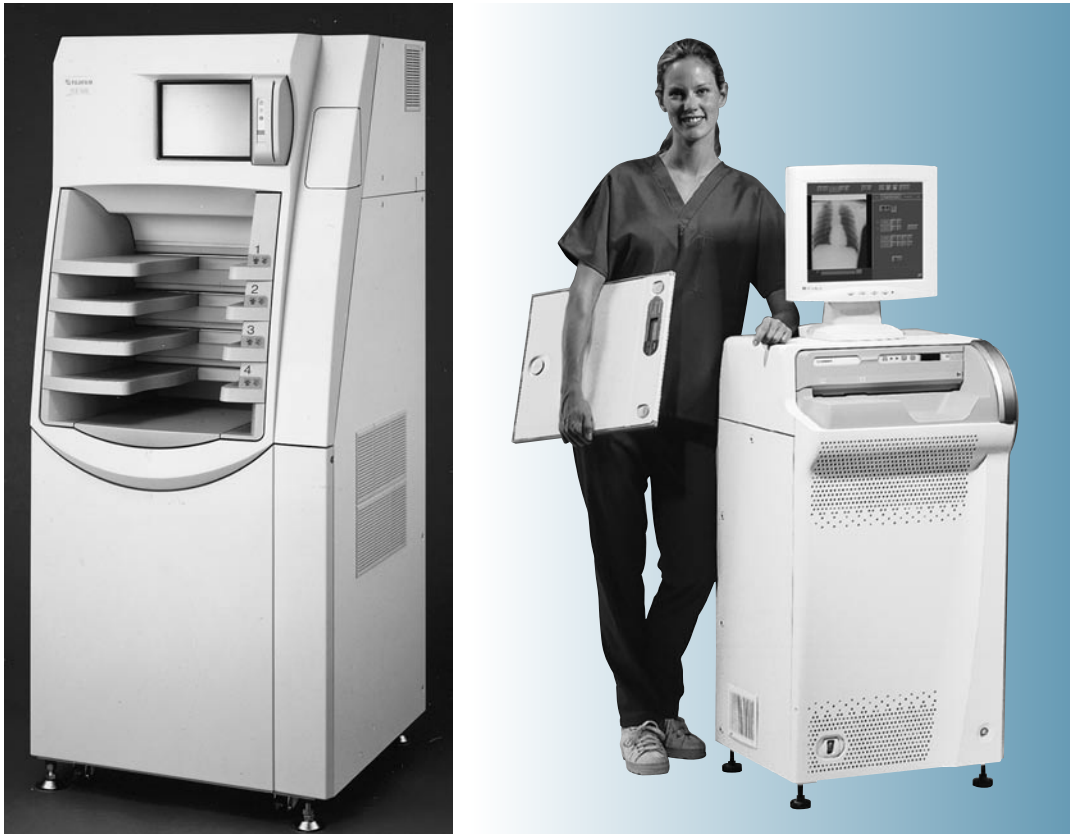
Figure 1-3 Examples of two CR readers. A , A high volume reader capable of processing between 110 and 140 imaging plates per hour. B , A much smaller system designed for medical offices, surgery, or intensive care units, capable of processing 50 to 60 imaging plates per hour.
