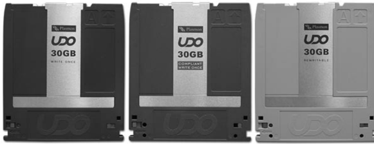
Figure 9-14 An ultra density optical (UDO) disk. (Courtesy Plasmon.)
