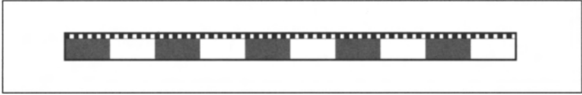
Figure 4.3. Measurement stick. (Here the stick is shown in a horizontal position; in the context of the water heights, the stick is positioned vertically.)
