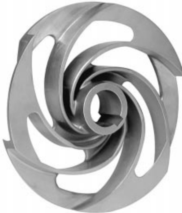
Fig. 18.3 Axial force-free impeller.
