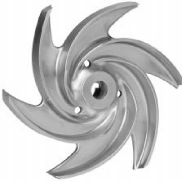
Fig. 18.2 Open impeller with compensation bores reducing the axial thrust.
