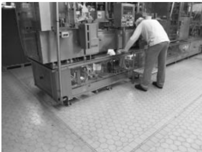
Fig. 15.6 Electrical equipment and valves below the machine in a visual and cleanable compartment 100 mm from the floor.
