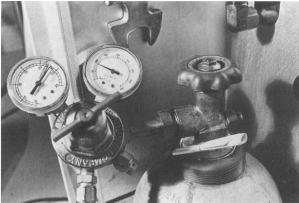
Figure 2.25. Gas pressure gauge and flow rate gauge.
