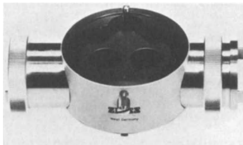
Figure 2. The beam splitter for the Zeiss microscope with two openings for attachment of accessories.
