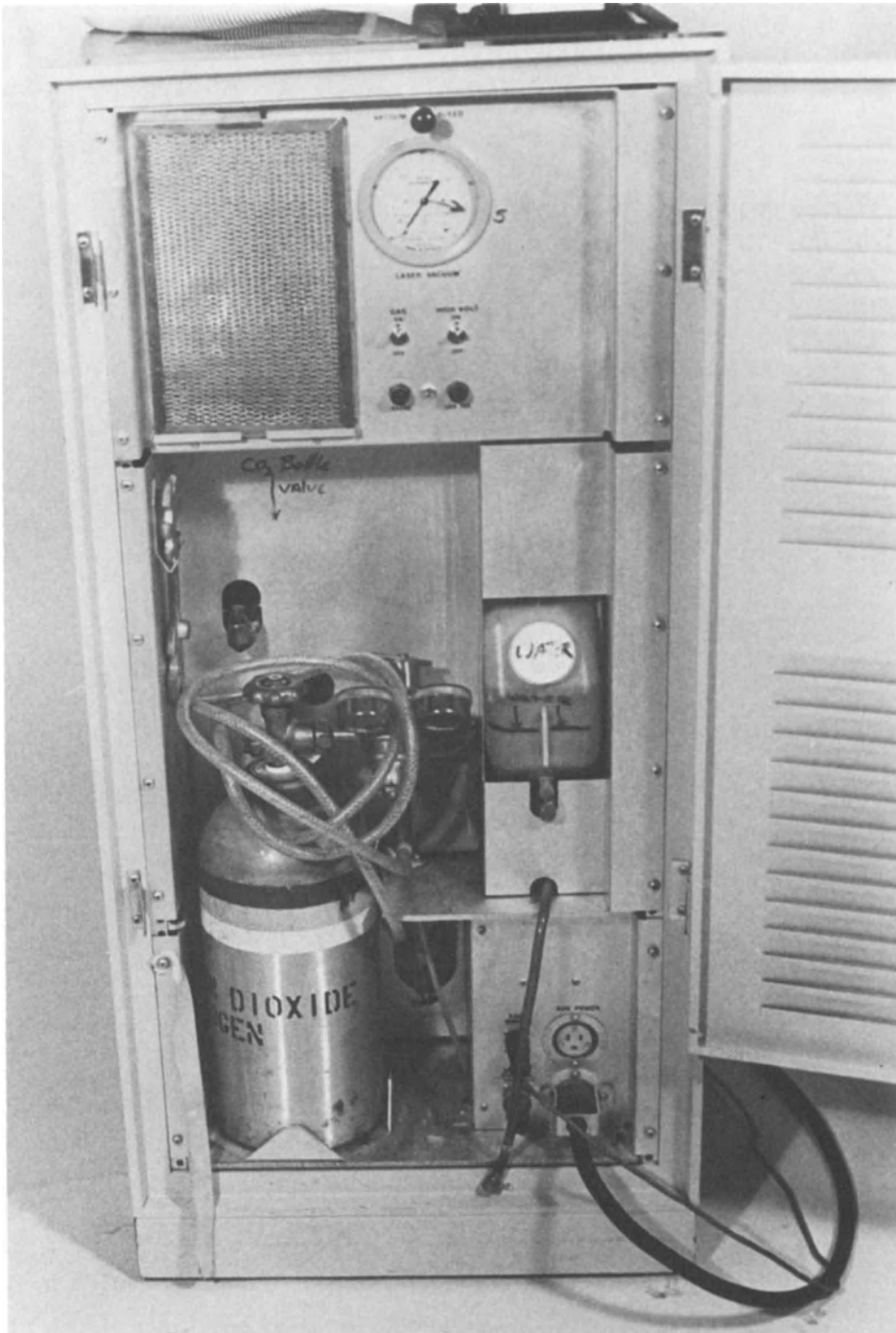
Figure 2.24. Access door to laser cabinet.
