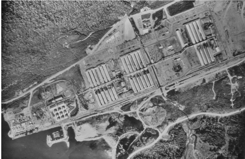
Aerial view of the layout of the Alcan aluminum smelter soon after it started production at Kitimat, British Columbia. Dock facilities for alumina, and aluminum shipments are in the foreground, and alumina storage silos are visible at the left end of the site.
