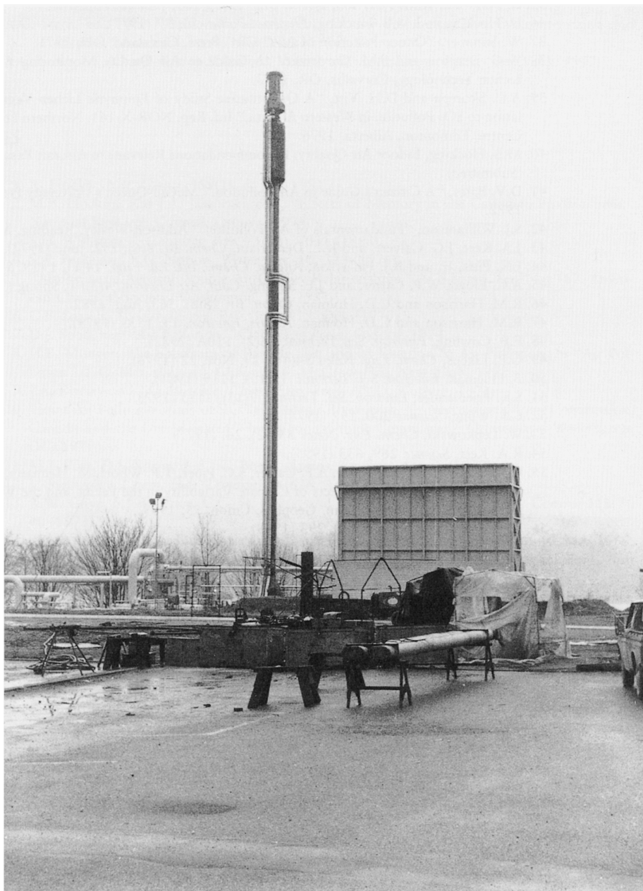
Oil refinery emergency flare for safe combustion of hydrocarbons during process upsets.
