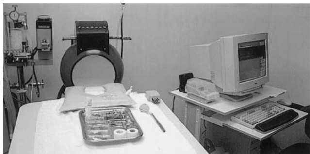
FIGURE 83.1 Computerized Ganzfeld ERG system for use in larger animals. Suitable adjunct utilities are demonstrated on the table: a deflatable cushion that aids in apposition of the head, a tray for electrodes, instruments used for stay suturing, and ophthalmic medications (methyl cellulose, phenylephrine hydrochloride, and atropine).
