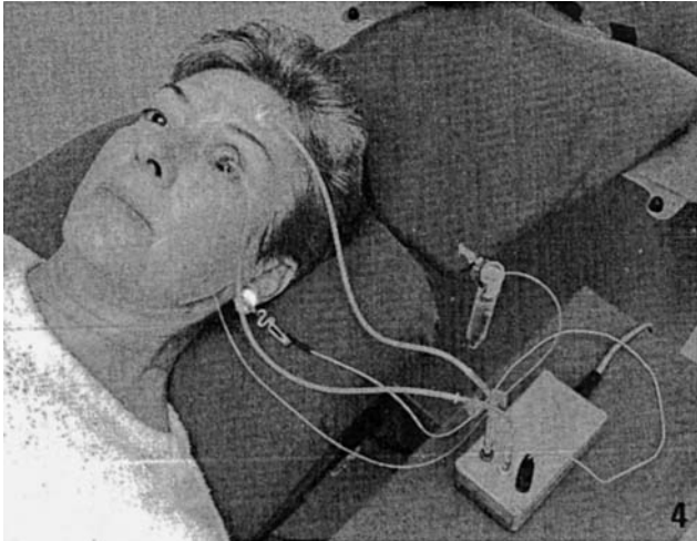
FIGURE 42.4 A contact lens on the eye and a plastic chamber on the forehead are connected by means of saline-agar bridges to matched calomel half-cells (recording and reference electrodes) plugged into a preamplifier. To provide a well-defined suction the contact lens is equipped with a second tube ending in a test tube with saline, the surface of which is located 20 cm below the eye. The earlobe is grounded. (From Nilsson SEG, Andersson BE. 26 Used by permission.)
