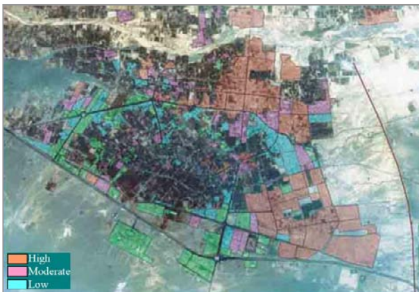
Figure 9: Bam buildings damage after earthquake (survey by JICA 2004).
