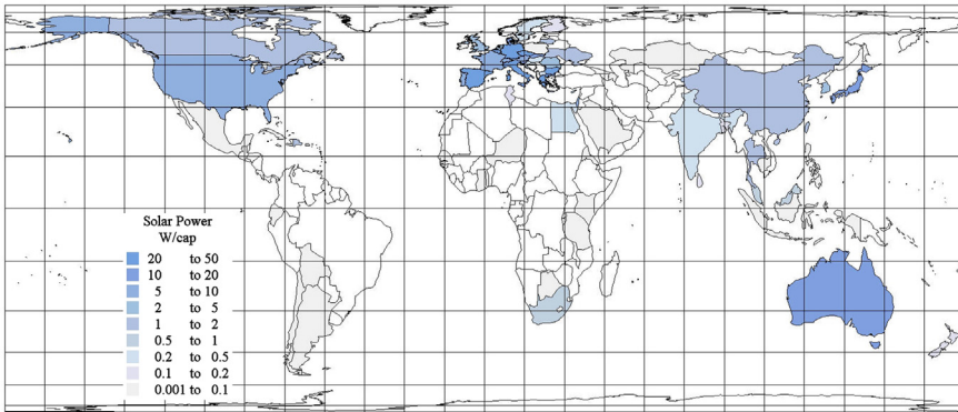
Figure 1.14 Solar power: National average values for the year 2013 (OECD, 2015). The world average for the year 2013 is 1.9 W/cap., up from 0.01 W/cap. in year 2000.
