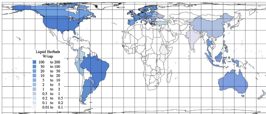
Figure 1.9 Energy in liquid biofuels (gasoline, diesel, or ethanol): National average values for the year 2013 (OECD, 2015). The world average for the year 2013 is 10.7, up from 2.3 W/cap. in year 2000.
