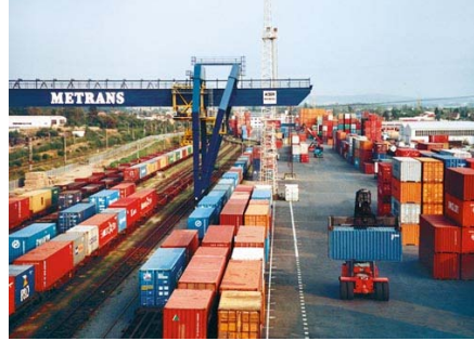
(b) Waiting trains under a gantry crane; a reachstacker on the right (courtesy of HHLA).
