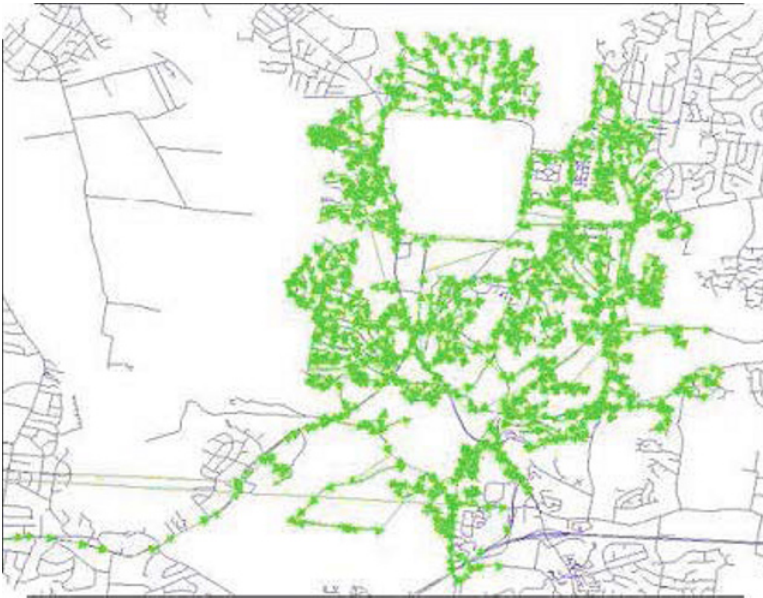
Fig. 3. Sample travel path for traversing each street segment.
