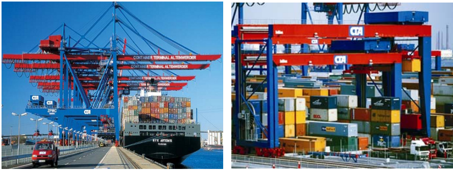
(a) Quay cranes (here: dual-trolley crane) serving a vessel (courtesy of HHLA). (b) Stacking cranes (here: DRMG) serving a container block in the yard (courtesy of HHLA).
