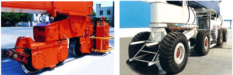
(a) Wheel of a RMG on rail (courtesy of Shanghai Zhenhua Port Machinery – ZPMC, www.zPMC.com). (b) Tire of a RTG (courtesy of ZPMC).
