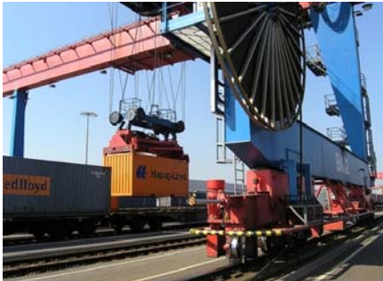
(a) Crane serving a train (courtesy of HHLA).
