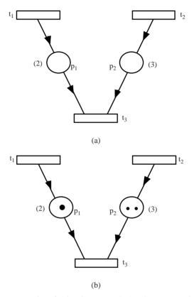
Fig. 7 Writing the state equation of a timed event graph. (a) The state equation for this example is  $x_3(n) \ge Max\{2+x_1(n);\ 3+x_2(n)\}$ . (b) The state equation for this example is:  $x_3(n) \ge Max\{2+x_1(n-1);\ 3+x_2(n-2)\}$
