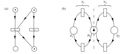
Fig. 5 Two characteristic examples of behavior that can be modeled using a Petri net. Fig.  $5(\mathbf{a})$  shows a situation of conflict between two transitions  $t_1$  and  $t_2$ : only one of these two transitions can be activated. Fig.  $5(\mathbf{b})$  shows an example of a situation of mutual exclusion where a common resource has to be shared between two subsystems  $S_1$  and  $S_2$
