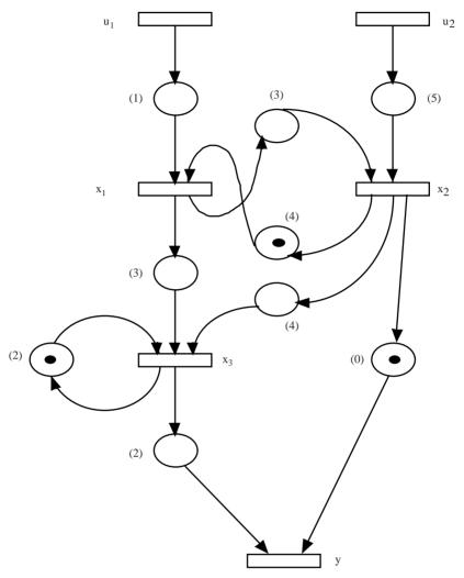
**Fig. 6** Example of a (timed) event graph. The time delays indicated between brackets next to each place, represent the minimal time a token has to stay in the place. We have also indicated the tokens in the initial labeling considered
