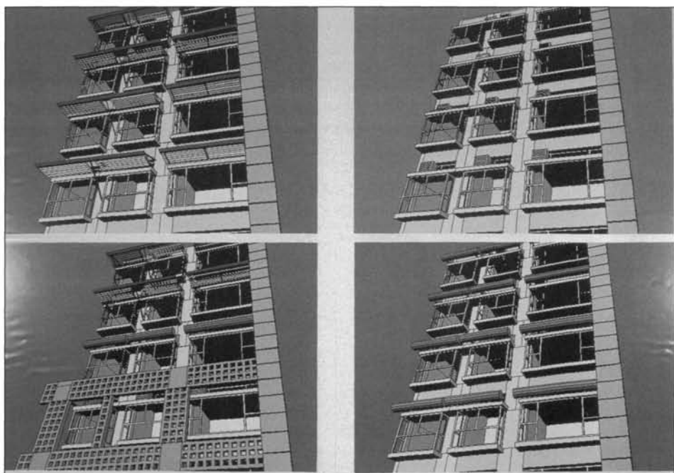
Plate 3 Solar-shading device: Study on alternative forms of external shading device.
