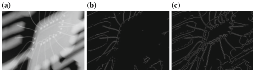
Fig. 3.2 Edge Detection in Image, a original image, b edge with the first derivative, c edge with the second derivative
