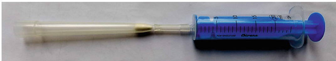
Fig. 3 5 mL sterile tip with inserted cotton wool connected with a short silicone tube to a 20 mL syringe used for additional filtration of the spore suspension
