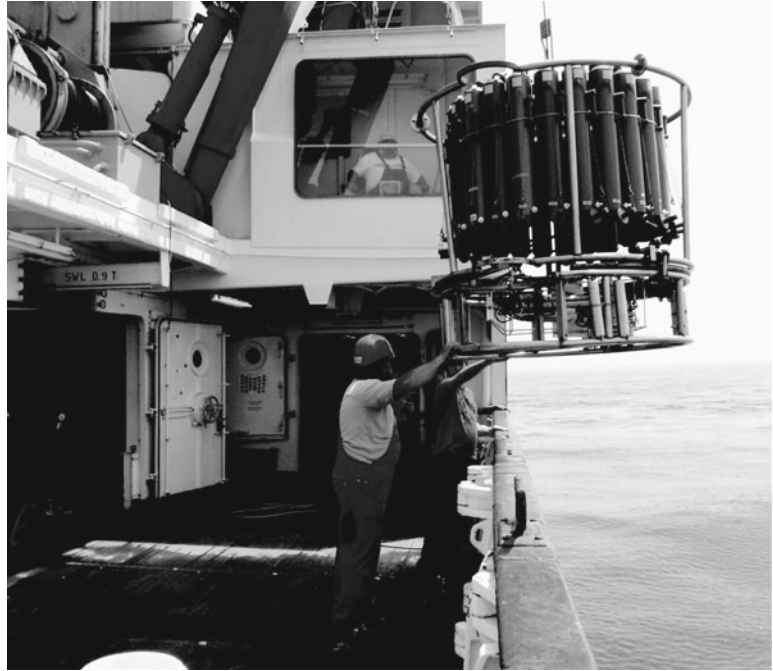
Fig. 1 CTD equipped with a 24 Niskin 10 L bottle rosette on German research vessel Meteor
