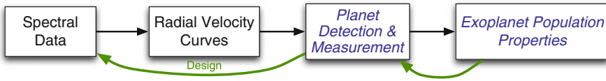
Fig. 42.2 Diagram of a discovery chain whereby exoplanets are found from periodic Doppler shifts in the spectra of the host stars. Progress in detection and characterization of individual planets leads to studies of exoplanet populations, and improved design of the observational experiments and spectral analysis procedures
