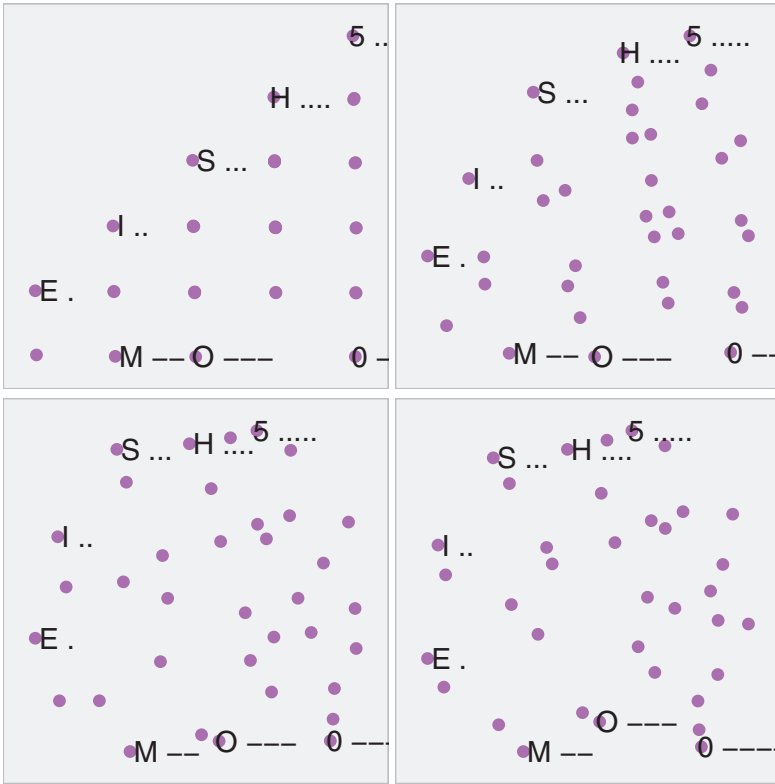
Fig. 6.12. Applying Kruskal–Shepard metric MDS scaling to the Morse Code confusion data: ( top left ) initial configuration, ( bottom right ) final configuration. Generally, codes of the same length are close to each other, as are codes with the same fraction of dots. The length of codes roughly increases from left to right, and the fraction of dots decreases from bottom to top.
