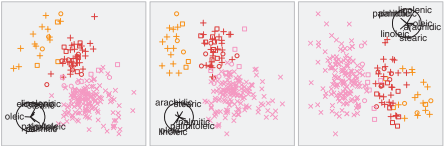
Fig. 4.15. Using the tour to examine the choice of support vectors when classifying Southern oils by area. Support vectors are open circles, and slack vectors are open rectangles; the data points are represented by +es and xes.
