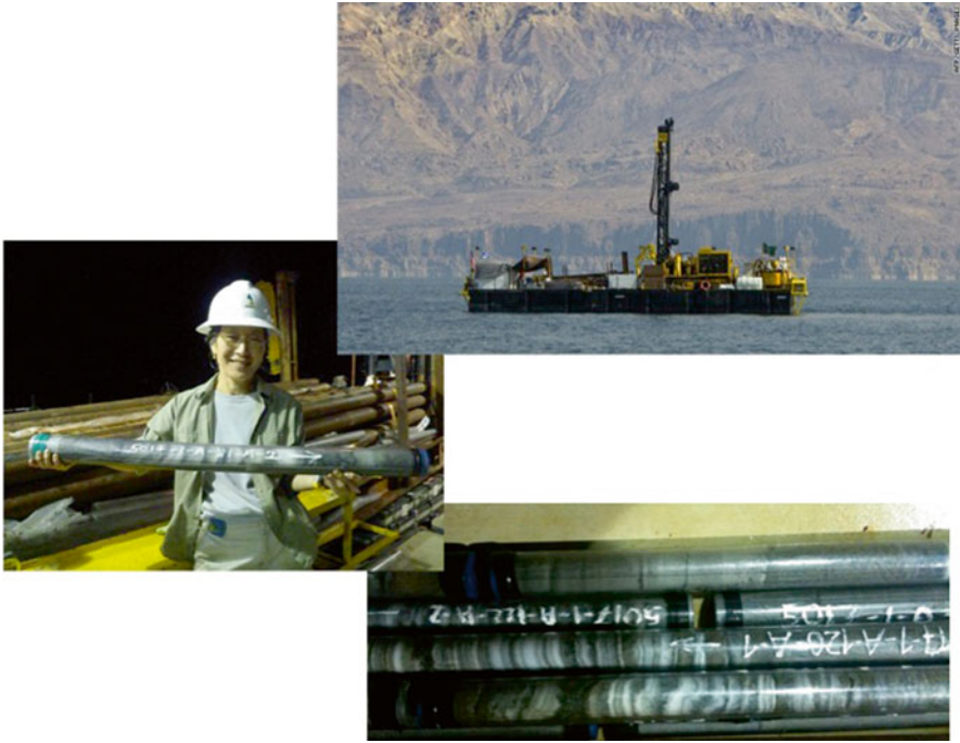
Fig. 10.14 Pictures from the ICDP Dead Sea drilling project (DSDDP) with DOSECC deep lake drilling facility. The displayed cores comprise sequences of marls and salt that were deposited during the last interglacial
