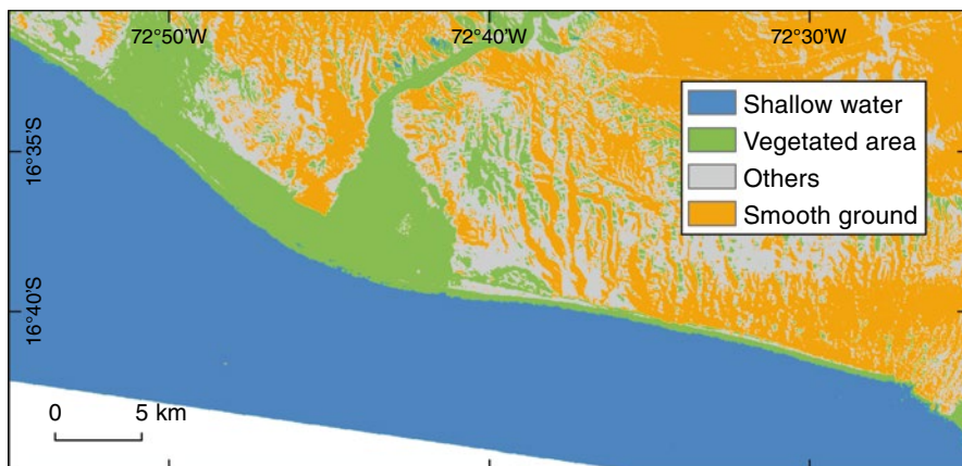
Fig. 1.6 Spatial distribution of roughness coefficient, according to the land-use condition, inferred from the unsupervised classification of pre-tsunami satellite imagery (Landsat-5 TM)
