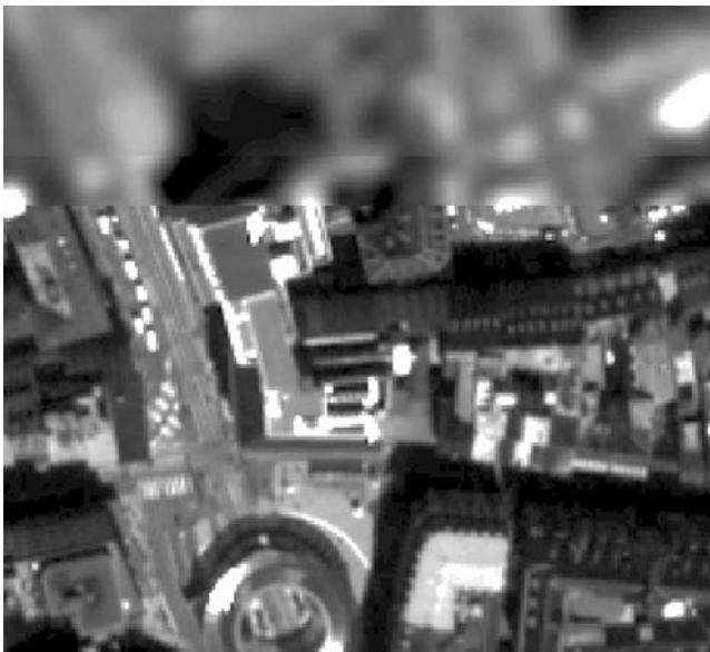
Fig. 11.4 Low resolution image with a high-resolution encrusted imagette with improved outer periphery
