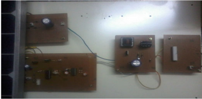
Fig. 50.13 Hardware setup of the cascaded DC to DC boost converter
