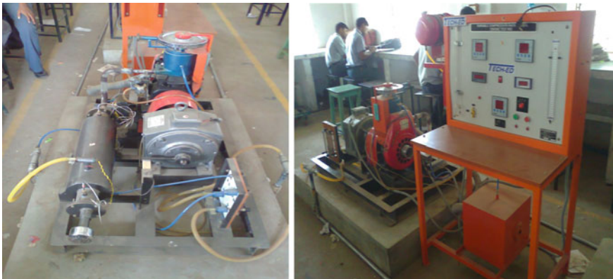
Fig. 3.1 Photograph of front and side view of SI engine experiment test rig
