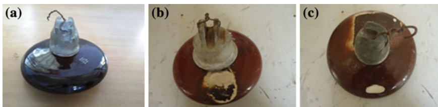
Fig. 132.2 Porcelain test insulators. a Without defect. b Defect near HV. c Defect far from HV. The disc type porcelain insulators with the range of 11 kV are involved in artificial pollution test
