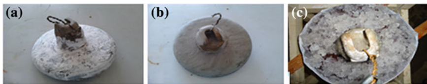
Fig. 132.3 a Coastal pollution on the surface of the porcelain insulator. b Industrial pollution on the surface of the porcelain insulator. c Polar pollution on the surface of the porcelain insulator
