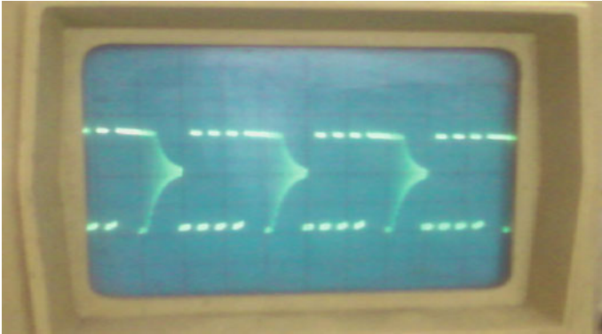
Fig. 105.12 Main winding voltage
