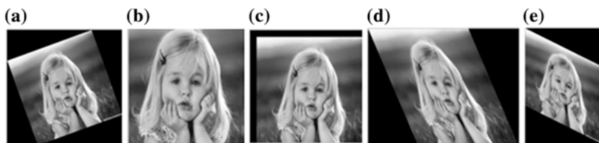
Fig. 119.3 Watermarked image subjected to various attacks. a Rotation, b Translation, c Scaling, d X-Shearing, e Y-shearing
