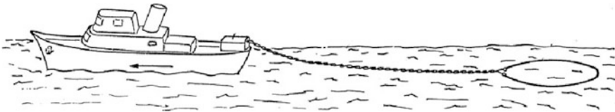
Fig. 1.16b Proposal (French patent) for a method for measuring the field with the aim of detecting the resistivity contrast of the underlying grounds (According to Duroux (1974))
