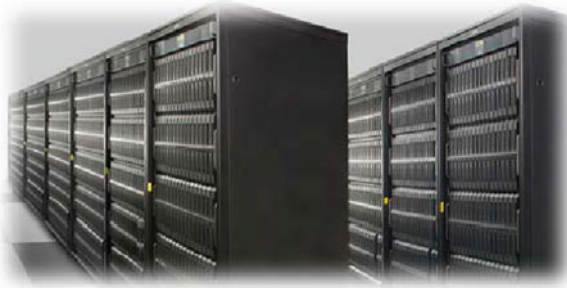
Fig. 5.3 Super computer used for processing, modeling and interpretation of electromagnetic data. Computing power (parallel computing) can handle today a very large number of data especially when used in the inversion process. These computers, such as Aurora of EMGS, are currently able to perform more than 70 trillion calculations per second
