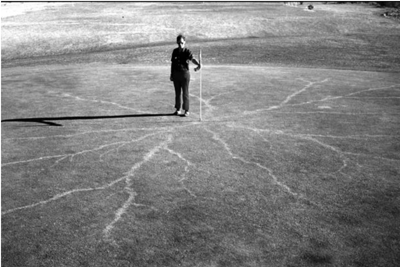
Figure 6.20 Evidence of surface arcing on a golf course green in Arizona (courtesy of E.P. Krider)
