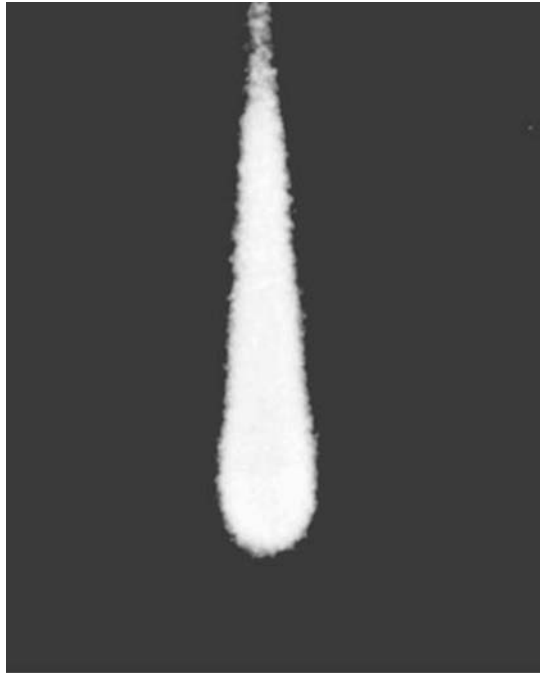
Figure 3.8 Cloud chamber photograph of a single electron avalanche (from [23])
