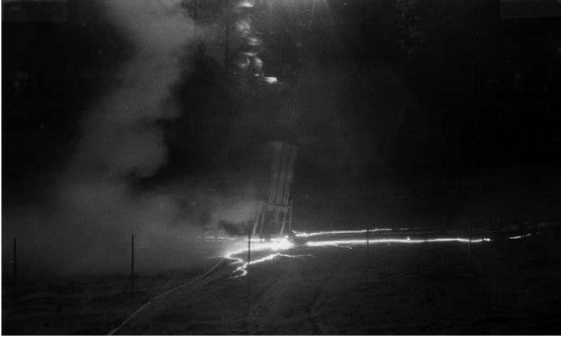
Figure 6.19 Photograph of surface arcing associated with the second stroke (current peak of 30 kA) of flash 9312 triggered at Fort McClellan, Alabama. Lightning channel is outside of field of view. One of the surface arcs approached the right edge of the photograph, a distance of 10 m from the rocket launcher (adapted from Fisher et al. 1994)
