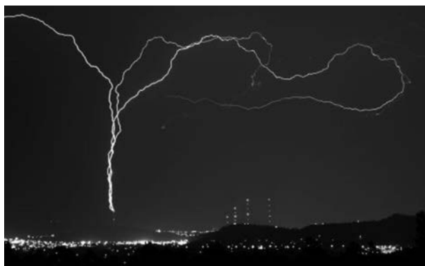
Figure 5.28 A composite image of three upward flashes photographed with a digital still camera (20 s exposure)
