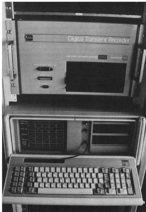
FIGURE 7.26 Digital transient recorder. (Courtesy of Rochester Instrument Systems Company, Rochester, NY.)
