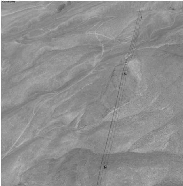
FIGURE 13.15 Selection of line route using Google Earth.
