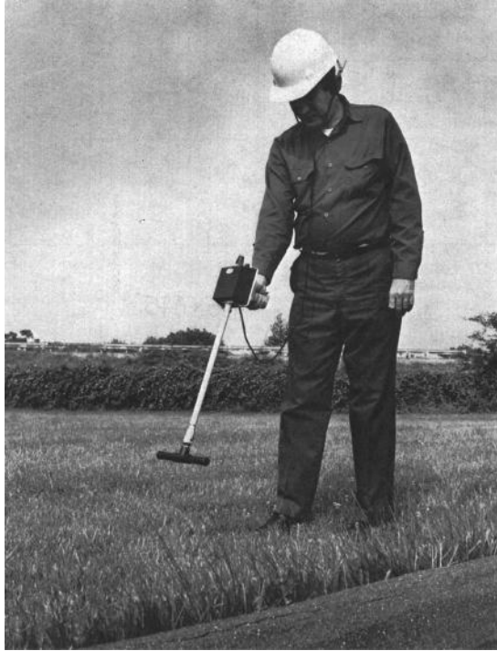
FIGURE 5.44 Lightweight battery-operated cable route tracer. (Courtesy of James G. Biddle Company, Philadelphia, PA.)
