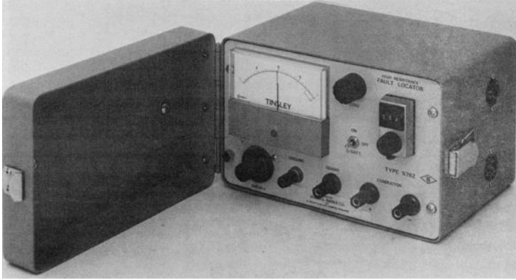
FIGURE 5.42 Portable Murray loop resistance bridge for cable fault-locating work. (Courtesy of James G. Biddle Company, Philadelphia, PA.)
